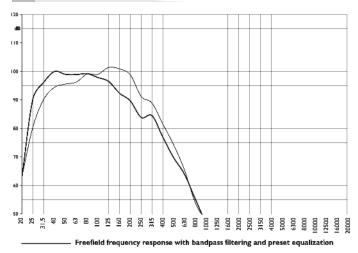
Freefield frequency response with bandpass filtering and no preset equalization
