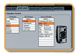
the sound engineer to apply different speaker models in real time from the comfort of the mixing desk. "Acoustic Integration" is the next live sound revolution.
